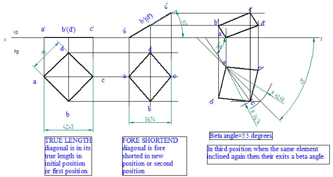
A square plane A, B, C, D of 30 mm sides resting onits corner such that the diagonal AC <u>appears to</u> be 45° to vertical plane and 30° to horizontal plane.
