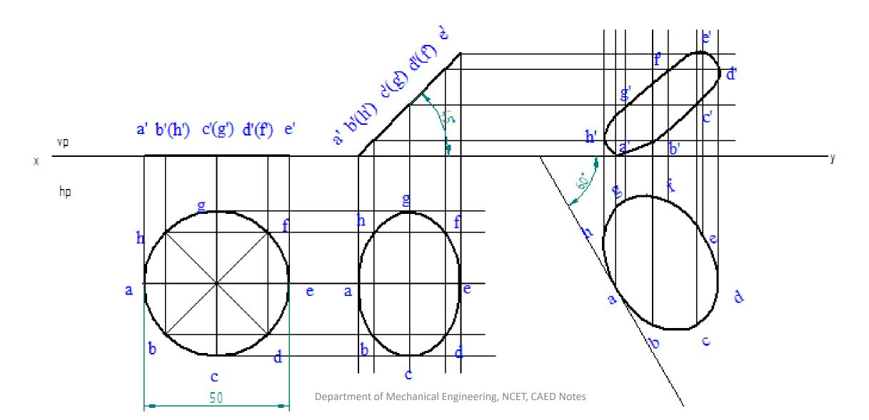
A square plane of 30 mm sides resting on horizontal plane such that one of the diagonal is inclined at 30° to horizontal plane and 45° to vertical plane on its corner, draw the projections.
