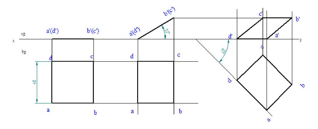
A rectangular lamina of sides 20 mm x 30 mm rests on horizontal plane on one of its longer edges. The lamina is tilted about the edge on which it rests till its plane surface is inclined to horizontal plane at 45°. The edge on which it rests is inclined at 30° to verticle plane. Draw the projections.
