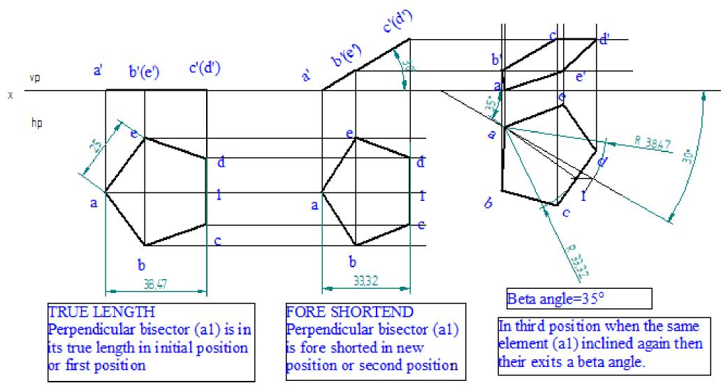
A pentagonal lamina of edges 25 mm is resting on horizontal plane with one of its corner such that the edge opposite to this corner is 20 mm above the horizontal plane and makes an angle of 45° to vertical plane. Draw the top and front views of the plane lamina in this posistion. Determine the inclination angle of horizontal plane.
