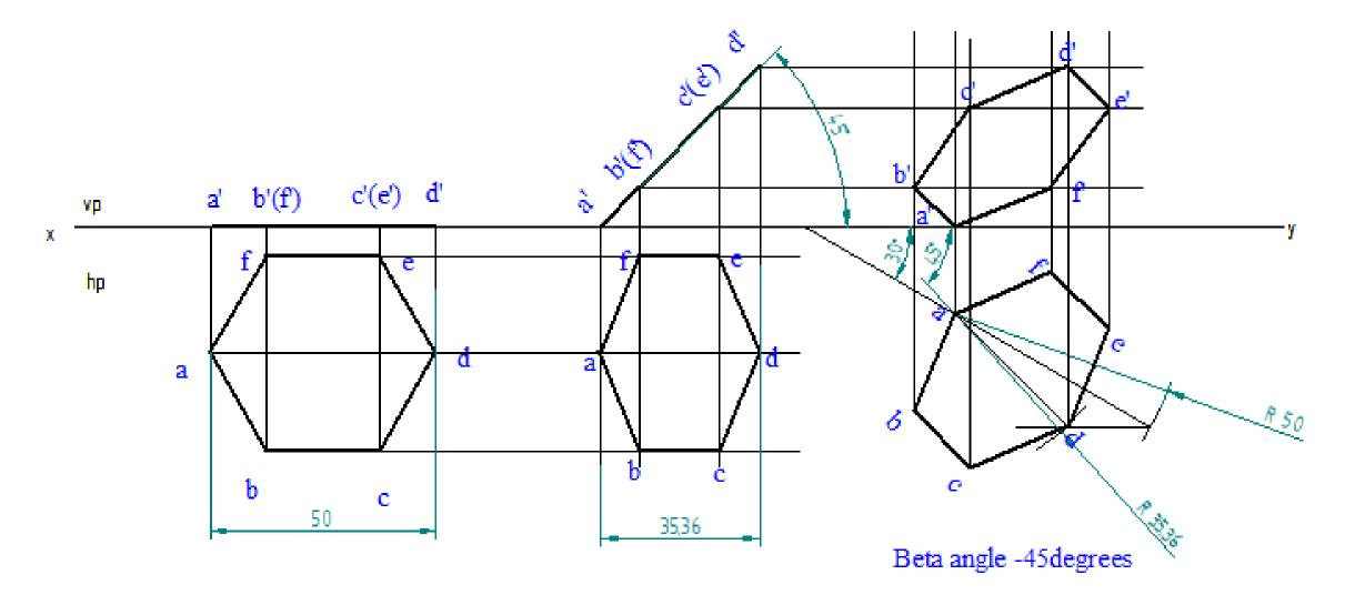
A pentagonal lamina having edges 25 mm is placed on one of its corner such that the perpendicular bisector passing through the corner on which the lamina rests it is inclined at 30° to horizontal plane and 45° to vertical plane.
